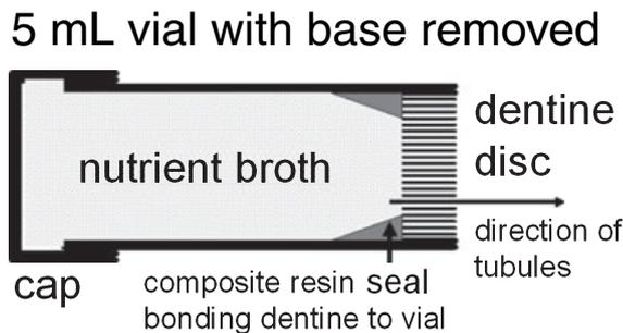
Fig 1. 5 mL vial showing the various components.
